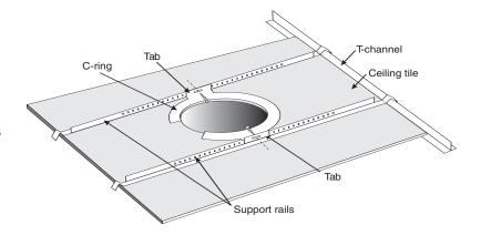
NOTE: If the rough-in bracket is used, it is not necessary to use the C-ring or support rails as shown in Step 2. Instead, in Step 5 below, use the doglegs to attach the speaker to the rough-in bracket instead of the C-ring.
